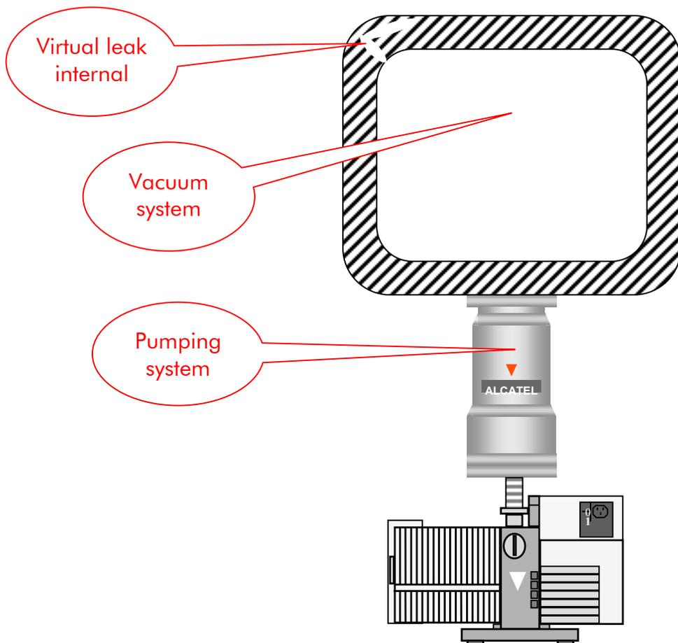
The virtual leak is also described as a gas load that comes out of the trapped volume during the pumping down phase.
