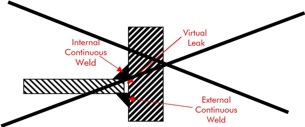
When two parts are welded together, there should be an internal continuous weld (on the vacuum side). There should be just a few welded spots on the outside for mechanical strength only. In the event both welds are continuous and a crack is present on the weld exposed to the vacuum side, the volume trapped between the two continuous welds will constitute a virtual leak.
