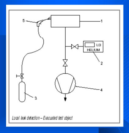
1 Test object 2 Leak detector 3 Search gas cylinder
