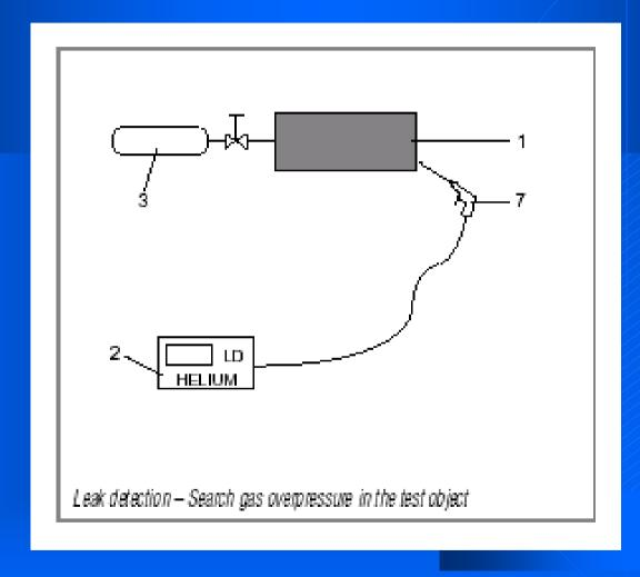
1 Test object 2 Leak detector 3 Search gas cylinder 7 Sniffer probe
