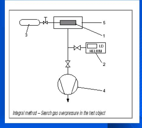
1 Test object 2 Leak detector 3 Search gas cylinder
