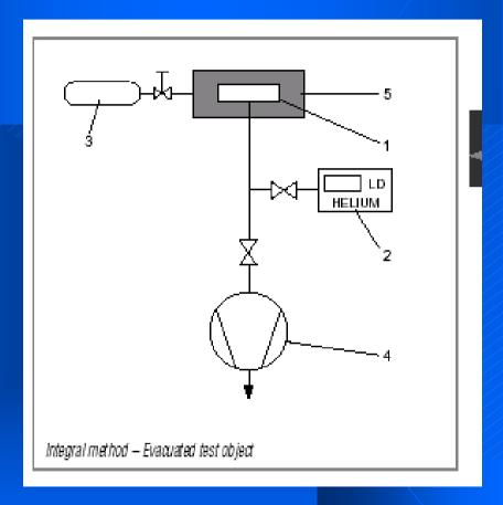
1 Test object 2 Leak detector 3 Search gas cylinder
